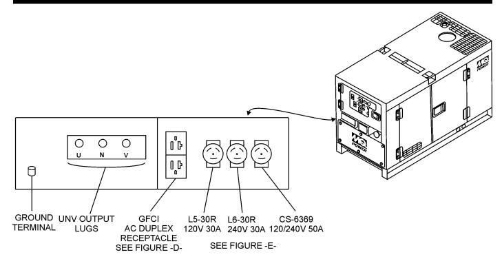
Figure 8. Receptacle Location on Generator
